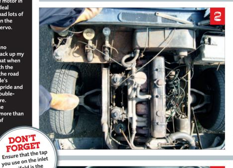
Find a suitable mounting position for the servo. Our RatSport item came with a mounting bracket. It must be far from direct sources of heat, like exhaust manifolds and never install it on the engine, drivetrain, suspension or anywhere subject to flexing or vibration. Follow fitment instructions referring to angles of installation that may come with your servo kit and ensure you're not about to destroy anything. Mark and drill relevant holes for attachment.
