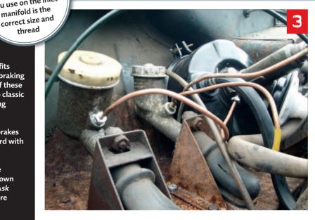
Begin the plumbing process by fabricating a length of brake pipe sufficient to reach from the brake master cylinder to the servo slave cylinder inlet port. Flare each end using a pipe former. Remember to fit the unions over the pipe beforehand. Be careful when bending brake pipes as kinks will restrict fluid flow and reduce braking efficacy. Use copper brake pipes (softer than steel), gradually bending them around a curved item of suitable diameter.
